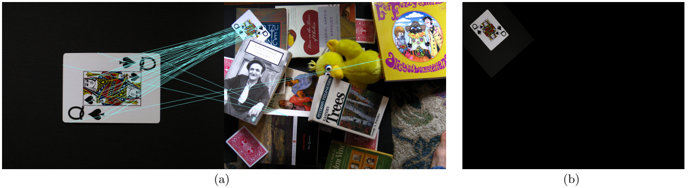
Figure 2: (a) Matches computed between SIFT keypoint in two images using the SIFT library’s kd-tree functions. (b) A transform computed between the two images based on the keypoint matches in (a) using the SIFT library’s RANSAC functions.
